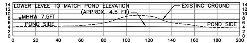
LEVEE REMOVAL – TYPICAL SECTION
