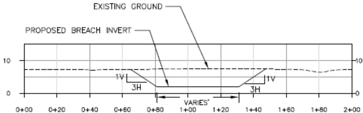
**Figure 4.5.** Proposed Levee Breach – Typical Section.
