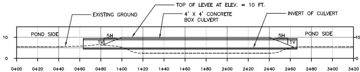
**Figure 4.9.** Proposed Water Control Structure – Typical Section
