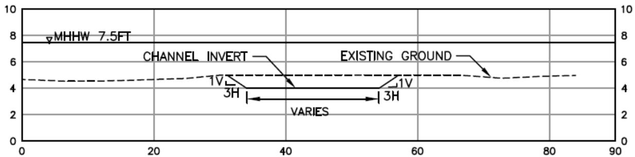
**Figure 4.7.** Proposed Pilot Channel – Typical Section.
