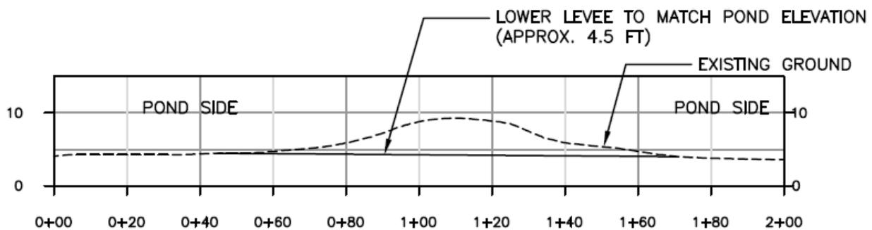
**Figure 4.4.** Proposed Levee Removal – Typical Section.
