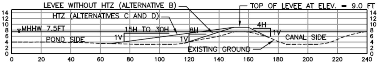
**Figure 4.2.** Proposed Levee Improvement – Typical Section.
