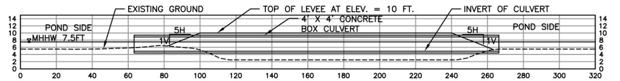
WATER CONTROL STRUCTURE – TYPICAL SECTION
