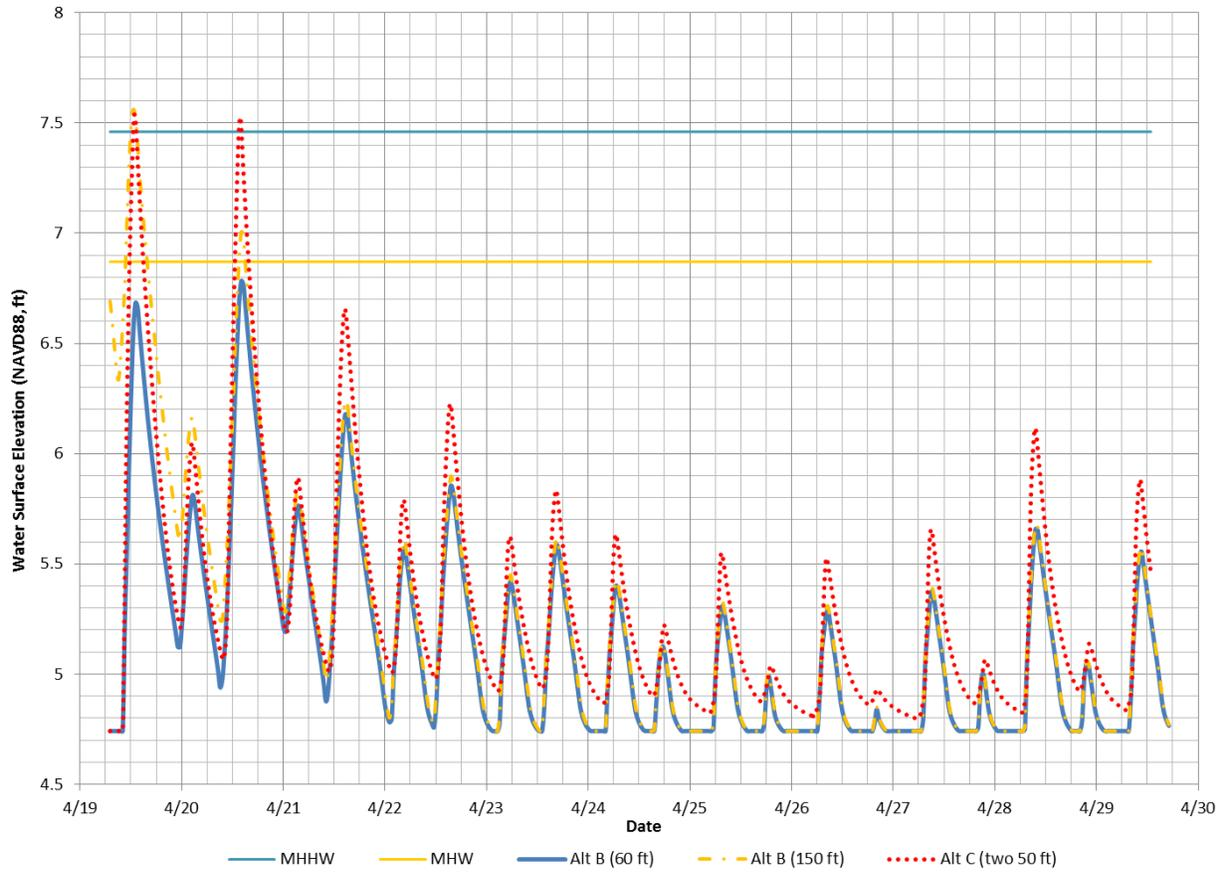
**Figure 3.7** Water surface elevations in Pond R4 at a point south of the main historical slough trace
