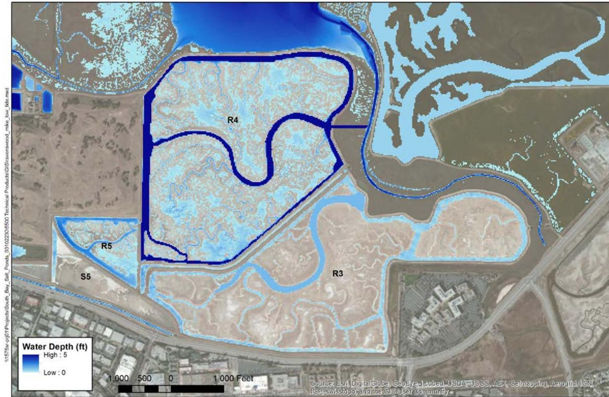
**Figure 3.8** Water depth during low tide for Alternative B with one 60-foot breach
