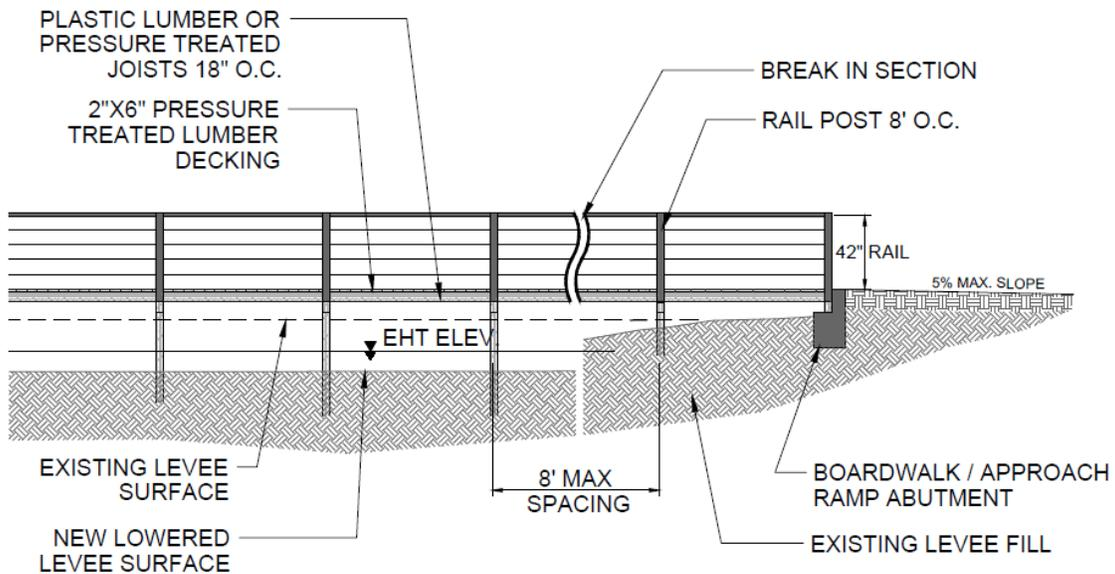
**Figure 4.11.** Proposed Boardwalk and Viewing Platform – Typical Profile
