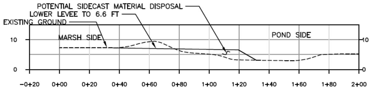
**Figure 4.3.** Proposed Levee Lowering – Typical Section.
