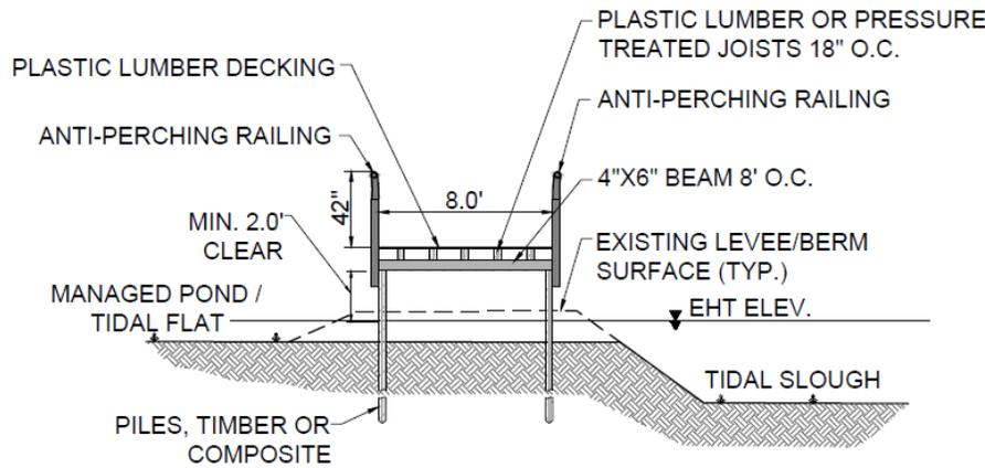
**Figure 4.10.** Proposed Boardwalk and Viewing Platform – Typical Section
