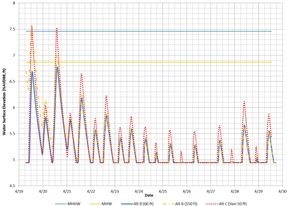
**Figure 3.6** Water surface elevations in Pond R4 at a point north of the main historical slough trace
