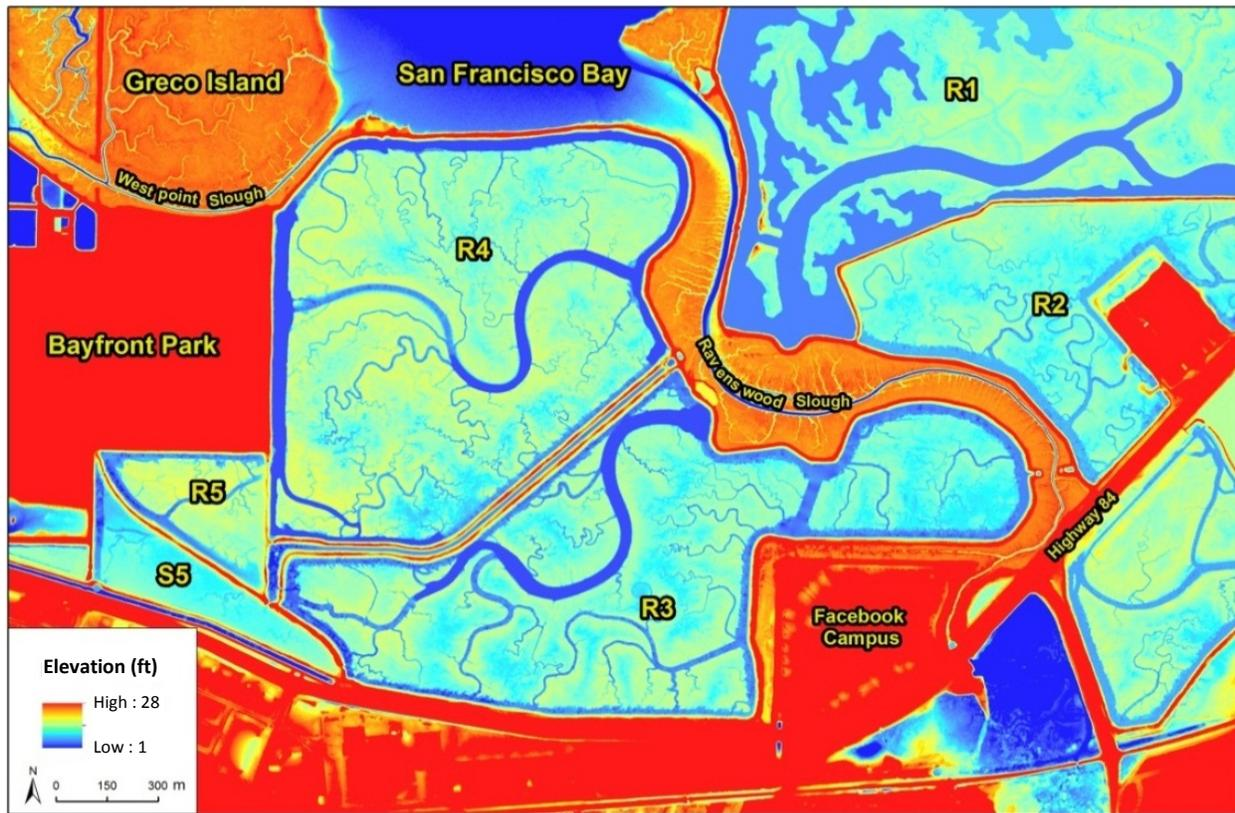
**Figure 3.2** Topographic and bathymetric map showing the ground surface elevations used to represent the Ravenswood Ponds and surrounding ground and water
